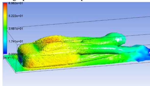
Figure 8. Vortex core region with velocity contour
