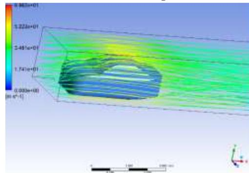
Figure 5. Velocity streamline on the car body
